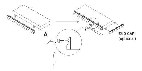
\* If END CAP will be installed replace the trim with the one supplied in the END CAP set F23C
